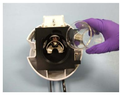
Figure 15 Filling the spray chamber
