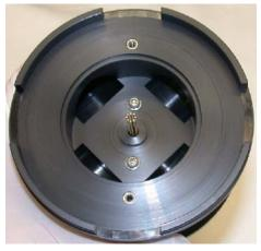
Figure 54 Octopole rods extending through Skimmer Spacer.
