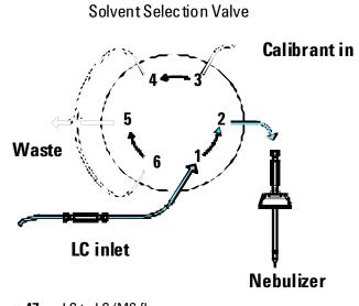
Figure 47 LC to LC/MS flow
