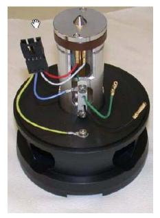
Figure 61 The re-assembled ion optics assembly
