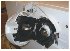
Figure 1 Opened electrospray spray chamber
