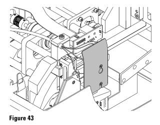
**10** Flip the stages assembly up and close the front pane.
