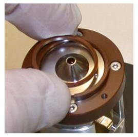
Figure 58 Spacer insulator
