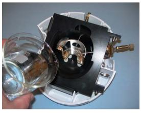
Figure 2 Filling the spray chamber
