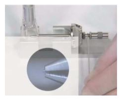
Figure 23 Adjusting the needle holder
