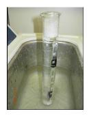
You may use a 1 mL pipette over the end of the ion transport capillary to protect the metallized plating. Trim the pipette tip to approximately 4 cm so that the capillary can be immersed in the cleaning solution.
