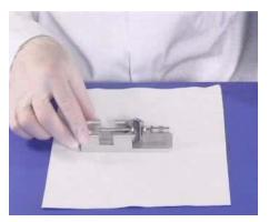
Figure 19 Electrospray nebulizer needle in needle holder
