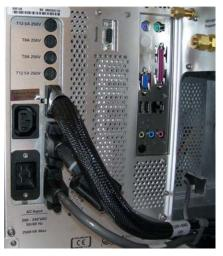
Figure 64 Disconnect the instrument power cable.
