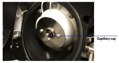
Figure 16 End of capillary cap
