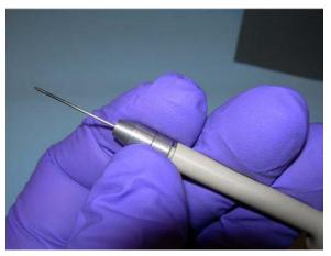
Figure 34 Unscrew the corona needle from the shaft.
