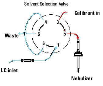
Figure 48 Calibrant to LC/MS flow
