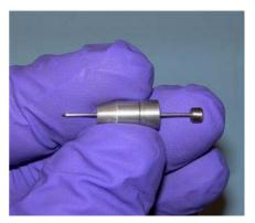
Figure 35 Replace the APCI corona needle.
