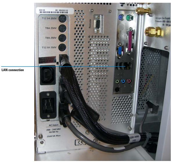
Figure 3 Connections behind service panel
