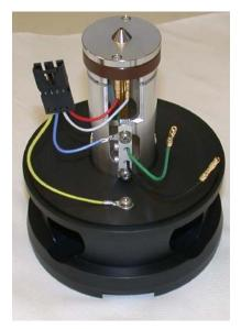
Figure 52 Ion optics assembly
