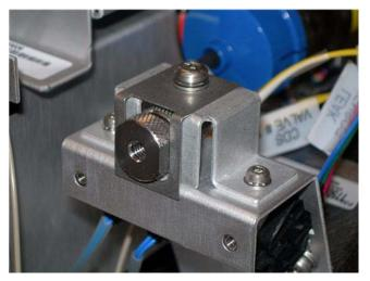
Figure 49 Inlet filter assembly
