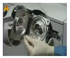
Figure 45 Reinstalling the capillary
