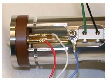
Figure 55 Lens 1 and Lens 2 wires
