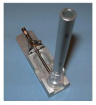
**Figure 6** Electrospray nebulizer needle in needle holder
