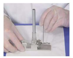
Figure 29 Installing the nebulizer in the adjustment fixture
