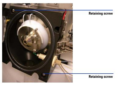
Figure 12 Remove the retaining screws. (6530 with IRM)
