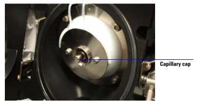
Figure 3 End of capillary cap
