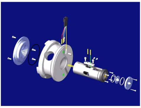
Figure 60 An exploded view of the ion optics assembly
