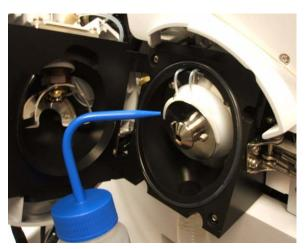
Figure 17 Rinsing the area around the spray shield
