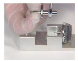
Figure 28 Tightening the union to compress the ferrule
