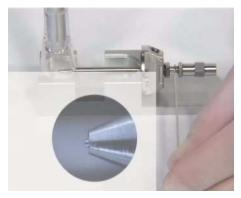
Figure 10 Adjusting the needle holder
