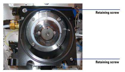
Figure 11 Remove the retaining screws. (6510 and 6520)
